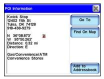
Use the Gas command in the Find 1 menu to locate the nearest gas station. The Nearest To Current Position screen (left) will appear. Scroll through the list and select a gas station. The POI Information screen (right) will appear. Select Go To and the unit will generate a route to the gas station.
